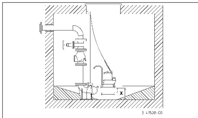
**Assembly:** Fix the coupling base firmly to the floor of the collection chamber using plugs and then mount the guide rails. Next, install the pressure pipe including the necessary fittings, such as the non-return valve and shut-off valves.
