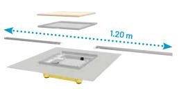
Quick and easy tiling works at line drainage because just one **one slope direction** is required. The channels themselves need a minimum slope to the center.
