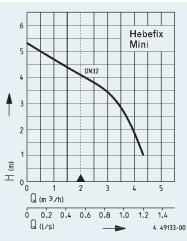
Powerful motor Hmax 5.3 m | Qmax 4.3 m<sup>3</sup>/h
